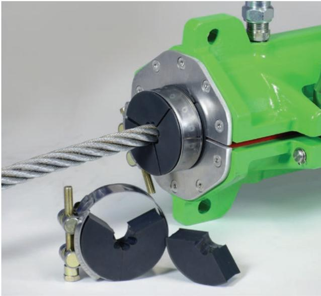
Viper Rope Cleaners enable the removal of contamination or built up old lubricant from the wire rope prior to lubrication, improving the effectiveness of the lubrication process via the Viper WRL. Viper Rope Cleaners (VRC's) are available in left and right hand lay, to suit 6 and 8 strand ropes and other strand configurations on request.
